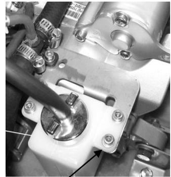
24. Coolant Expansion Tank Cap
